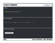
**How to update the system firmware** The downloaded file is extracted to a USB key which is then plugged into the surface for the update to be performed. The MixRack, Surface and TouchScreen are all updated at the same time.
